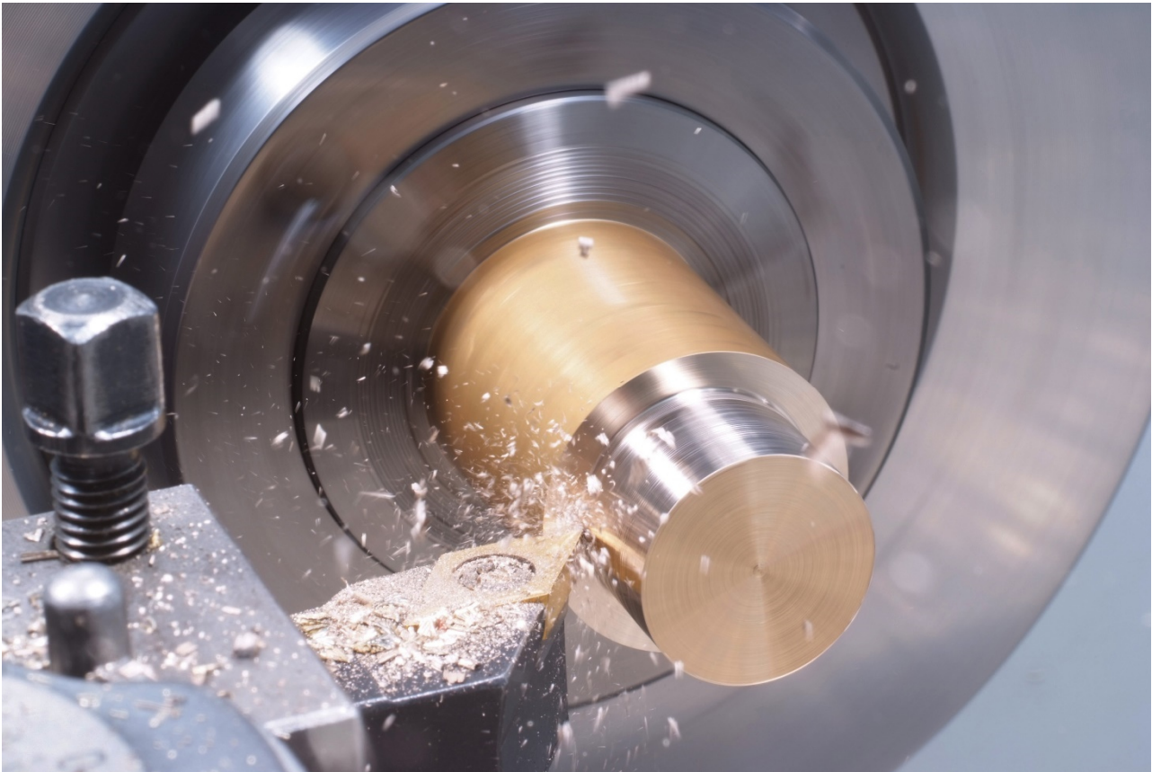
Machining lead-free brass rod at Wieland in Ulm - Photo courtesy of Wieland Group
