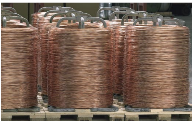
Wire wound onto uncoiling devices
