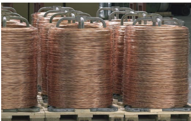
Wire wound onto uncoiling devices
