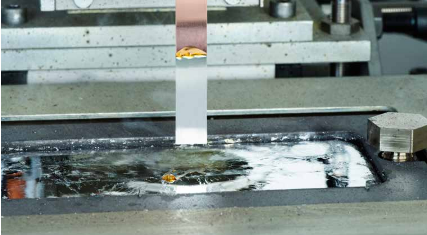
Solderability test according to DIN EN IEC 60068-2-20
