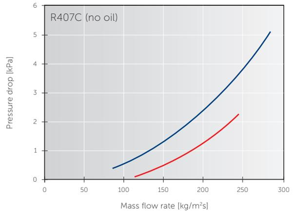
**Test conditions** Evaporation – 9.52 mm tubes  $t_c = 0\text{ }^\circ\text{C}$  superheat  $\sim 5\text{ K}$ , inlet quality 20 % tube length 2 m
