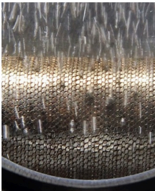
Figure 7. Boiling at 0 °C of propane with 0.16 K wall superheat on Wieland enhanced boiling tube (GEWA-PB).
