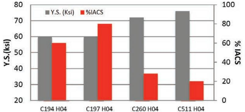
Figure 1: Comparison of Tensile Strength and Electrical Conductivity performance of select connector materials
