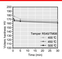
Vickers hardness after heat treatment (typical values)
