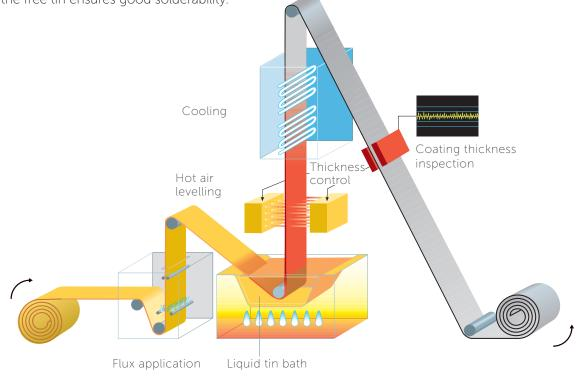
Fig. 1: Schematic of hot-dip tinning process
