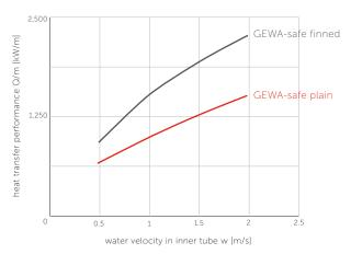
Test conditions: tube-in-tube measurement, media: annulus space water @ w=1 m/s, inside tube water, dT=10 K, outside diamter=19.05 mm, tube length=1 m
