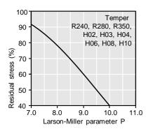
Stress remaining after thermal relaxation as a function of Larson-Miller parameter P (F. R. Larson, J. Miller, Trans ASME74 (1952) 765–775) given by:  $P = (20 + log(t))^*(T + 273)^*0.001$ . Time t in hours, temperature T in °C. Example: P = 9 is equivalent to 1,000 h/118 °C. Measured on rolled to temper specimens parallel to rolling direction. Total stress relaxation depends on the applied stress level. Furthermore, it is increased to some extent by cold deformation.
