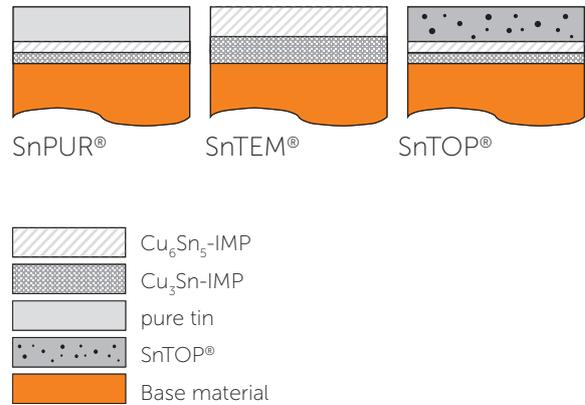
Fig. 2: Structure of hot-dip tin layers on copper alloys
