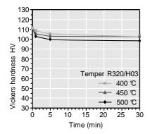
Vickers hardness after heat treatment (typical values)
