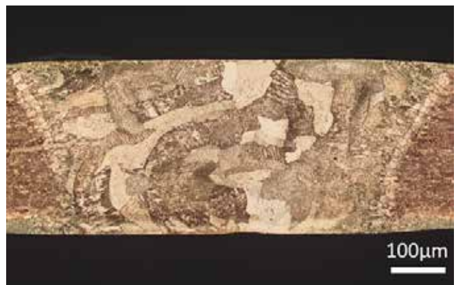
Figure 10 – TIG weld without filler material in Wieland-K65 TIG welds are mostly used as temporary welds to connect two strips before further processing and thus serve to reduce set-up times and increase the productivity during punching and coating. The transfer welds are removed after the stamping or coating processes. TIG weld seams are rarely/not used as joints in an electronic component itself.
