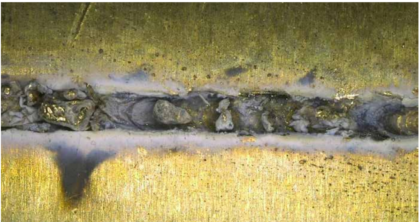
Figure 19 – Laser weld in CuZn37
