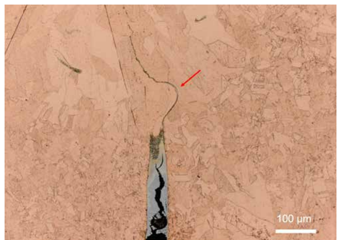
Figure 20 – Tin streaks in a seam root after welding of tin coated pure copper
