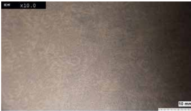
K65; 0.32mm; 1–2µm tin layer thickness; SnTEM
