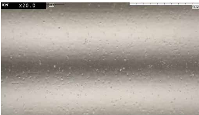
K73; 0.246mm; 1–3µm tin layer thickness; SnPUR
