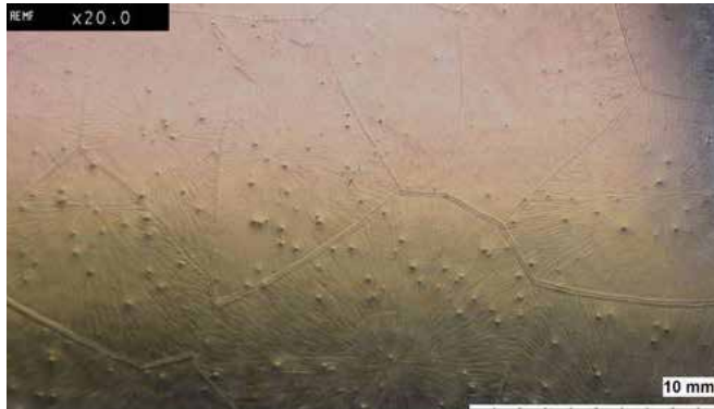
K55; 0.8mm; 10–18 \mu\text{m} tin layer thickness; SnPUR
