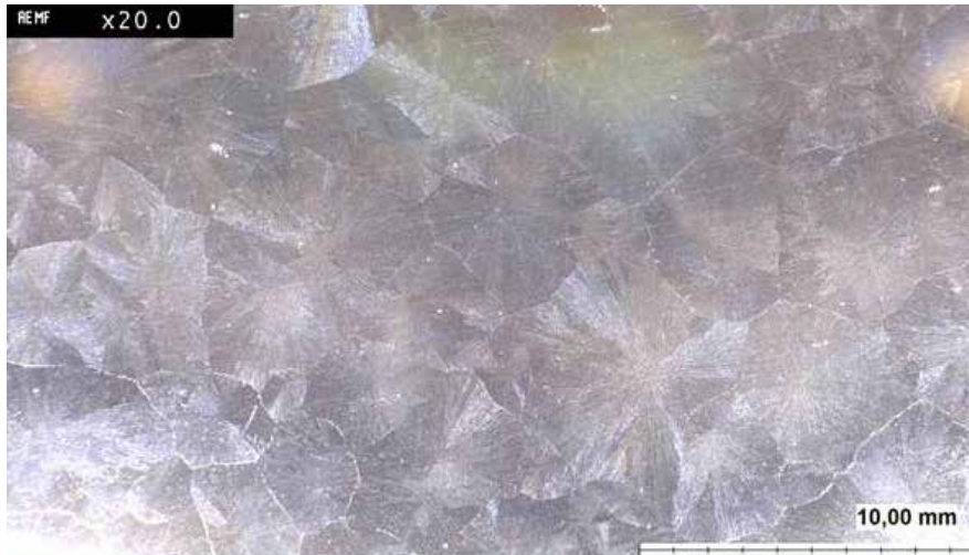
K81; 0.2mm; 1–3 \mu\text{m} tin layer thickness; SnTOP
