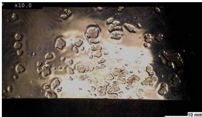
K62; 0.3mm; 4–8 \mu m tin layer thickness, SnPUR
