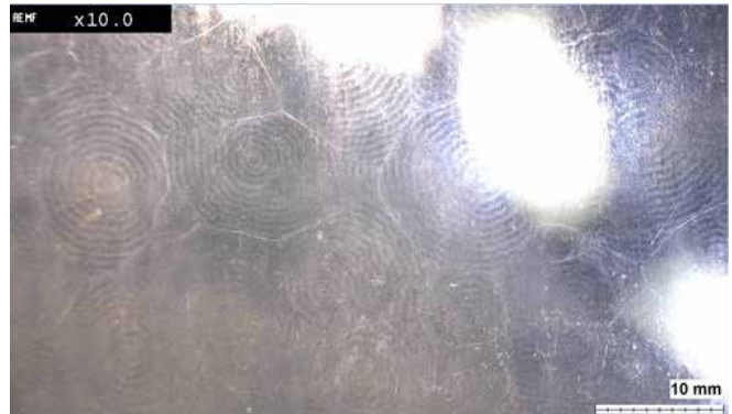
Thick tinning with typical circular structure
