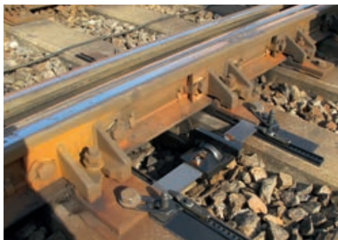
Austroroll MFR in a retrofit version.
