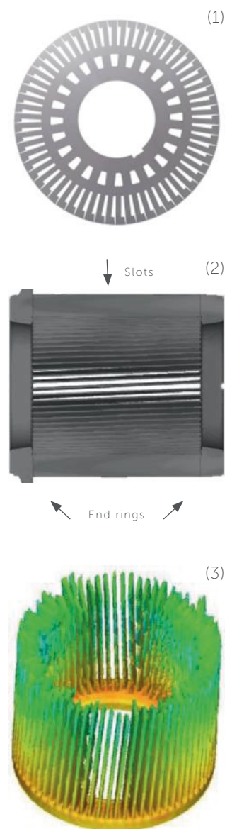
Fig. 1: Electrical steel sheet, cast squirrel-cage (consisting of the first and second end ring, connected by conductor rods); manufactured via casting process, shown here: Laminar Squeeze Casting.
