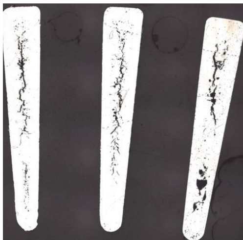
Fig. 4: Micrographs of the slots and end rings of the rotor in the conventional casting process [3,4].
