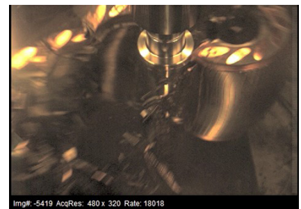
Fig. 10: burst test, ZPR® copper rotor, single frame video recording at 27,614 \text{ min}^{-1} and a circumferential speed of 205.6 \text{ m/s} .
