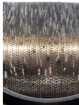
Figure 6: Boiling at 0°C of propane with 0.16K wall superheat on Wieland enhanced boiling tube (GEWA-PB)
