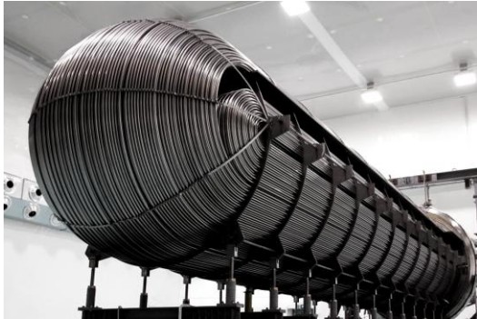
Heat exchanger for nuclear power plants manufactured by Neotiss
