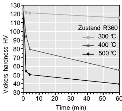
Vickers hardness after heat treatment (typical values)
