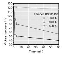
Vickers hardness after heat treatment (typical values)
