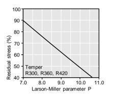
Stress remaining after thermal relaxation as a function of Larson-Miller parameter P (F. R. Larson, J. Miller, Trans ASME74 (1952) 765–775) given by:  $P = (20 + log(t))^*(T + 273)^*0.001$ . Time t in hours, temperature T in °C. Example: P = 9 is equivalent to 1,000 h/118 °C. Measured on rolled to temper specimens parallel to rolling direction. Total stress relaxation depends on the applied stress level. Furthermore, it is increased to some extent by cold deformation.
