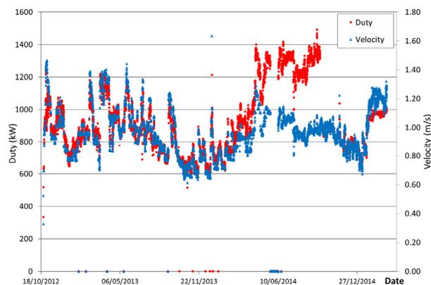
**Figure 3:** Heat exchanger duty and quench water velocity profiles
