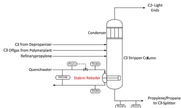
**Figure 1:** C3 Stripping unit with stab-in HEX and instrumentation
