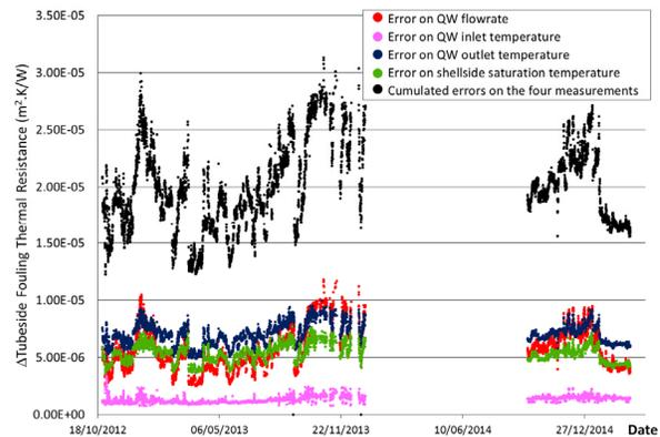
**Figure 8:** Impact of measurements accuracy on tubeside fouling thermal resistance
