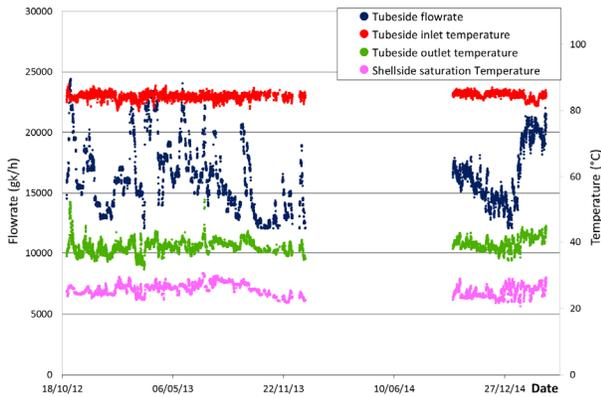
**Figure 6:** Filtered recorded data over the 2 years operation, calculated with *Edgeview* – quench water inlet & outlet temperatures, quench water flowrate and C3 saturation temperature
