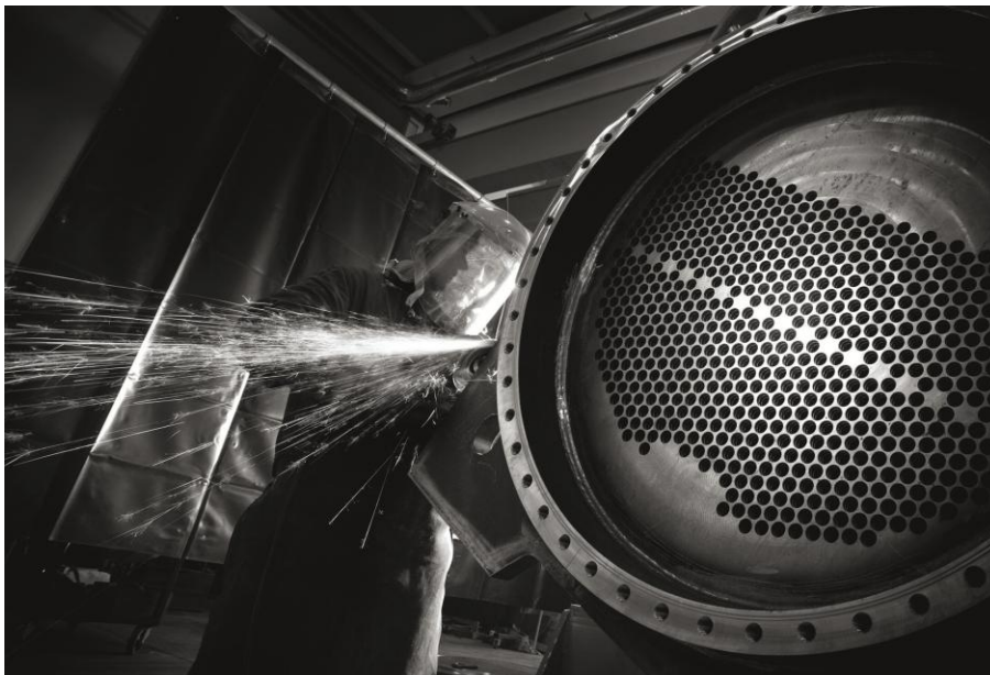
Manufacturing heat exchangers at Wieland’s facility in Delaware, Ohio.
