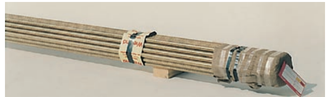
Bundle of round rods \geq 10 mm Bundle of sections/tubes Weight: 1000 kg (500 kg)
