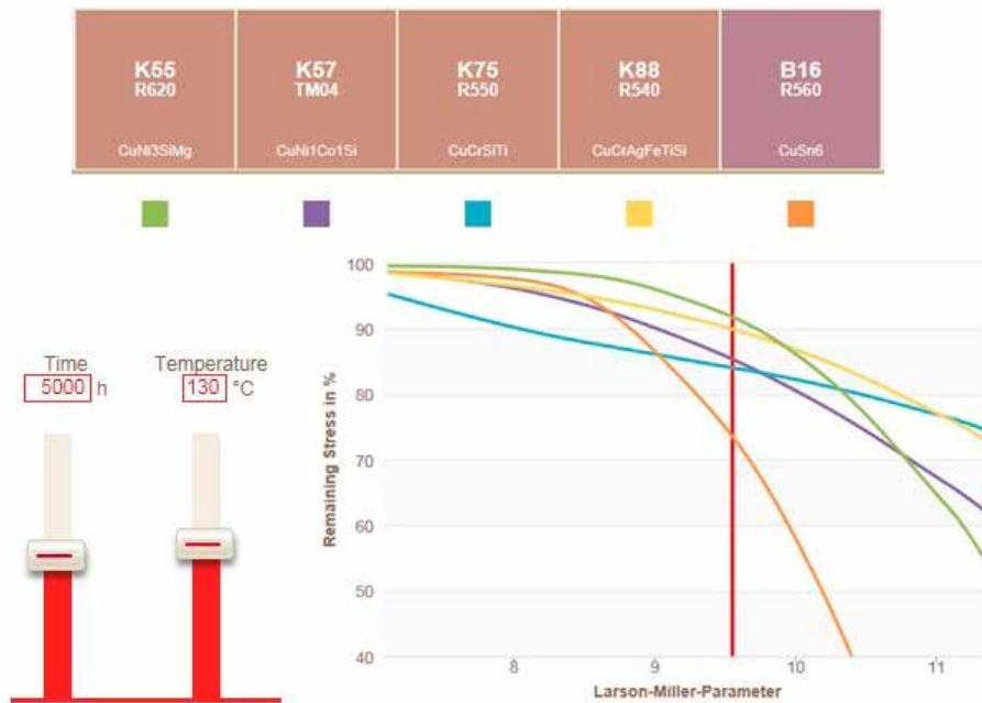
Fig. 4: Thermal stress relaxation diagram of high performance alloys in comparison with phosphor bronze.
