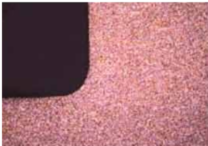
Micrograph section of a milled profile strip: the structure of the base material is the same
