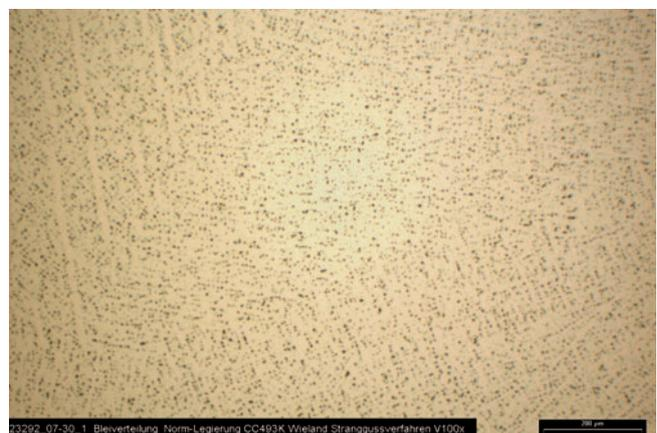
Lead distribution of the same standardised alloy CC493K, however, manufactured using the Wieland continuous casting process (with 100x magnification, Wieland-G07)
