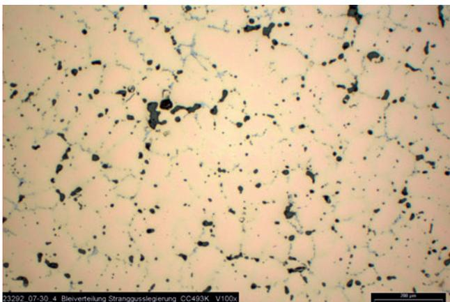
Lead distribution of a conventional continuous cast alloy (with 100x magnification; alloy CC493K)
