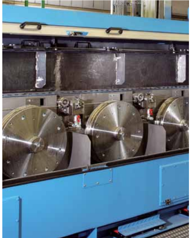
The wire is manufactured on state-of-the-art drawing lines equipped with diamond drawing tools, computer-controlled drives, multiple draws, an in-line annealer as well as optimised lubricant technology.
