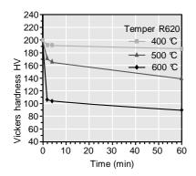
Vickers hardness after heat treatment (typical values)
