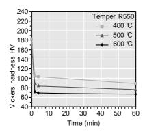
Vickers hardness after heat treatment (typical values)
