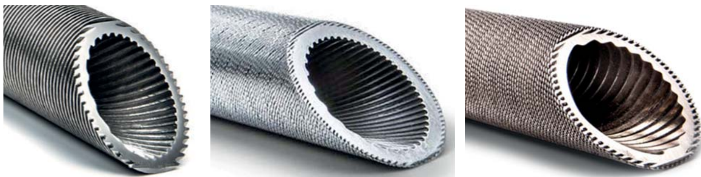
Figure 1. GEWA dual-enhanced heat exchanger tubes. (a) GEWA-KS, with fins on both sides, (b) GEWA-PB, with boiling enhancement outside (c) GEWA-CLF (Low Fouling), with condensing enhancement outside. Images courtesy of Wieland.
