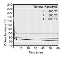
Vickers hardness after heat treatment (typical values)
