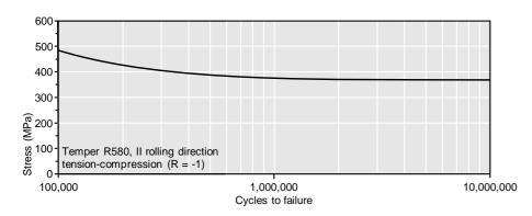
The fatigue strength is defined as the maximum bending stress amplitude which a material withstands for 10<sup>7</sup> load cycles under symmetrical alternate load without breaking.
